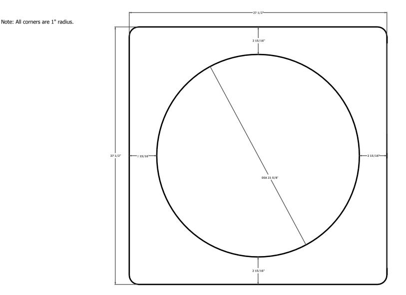
NOTE: Before cutting fan hole, measure the inner fan shroud diameter to make sure that there is enough lip for it to sit securely and firmly on the plywood. Adjust hole diameter as needed. Different fans models make require modifications to diameter to fit.
